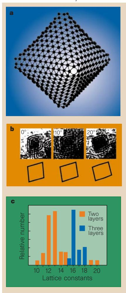
**Figure 1** Structure of the molecules. **a**, Model octahedron with an edge length of 12 *a* lattice constants showing only the molybdenum sublattice. **b**, Transmission electron microscope images and model-generated projections for a three-layer  $\text{MoS}_2$  rhomboid at 0° and undergoing tilts of 10° and 20°. **c**, Histogram of octahedral edge lengths in *a* lattice constants determined from 30 rhomboidal, rectangular and hexagonal projections observed by TEM.
